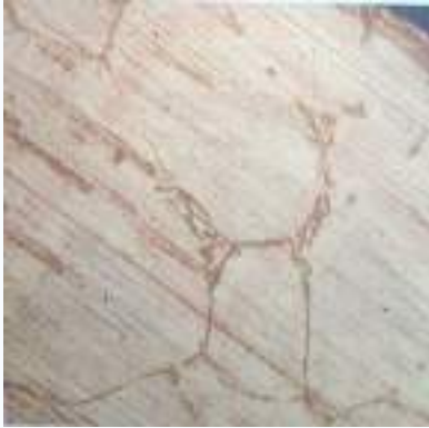
Figure 8 Microstructure of the specimen without vibration.
