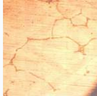
Figure 9 Microstructure of the specimen with vibration.
