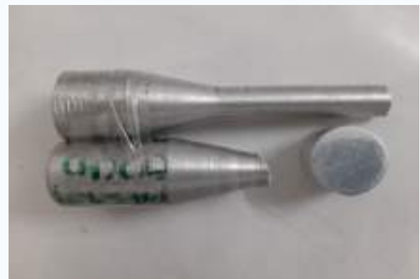
Figure 6 Specimen without vibration casting after testing.
