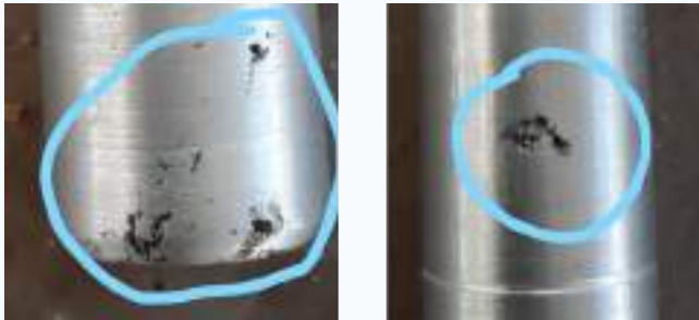
Figure 4 Defects on the specimen without vibration casting.
