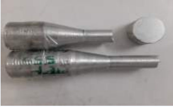
Figure 7 Specimen with vibration casting after testing.
